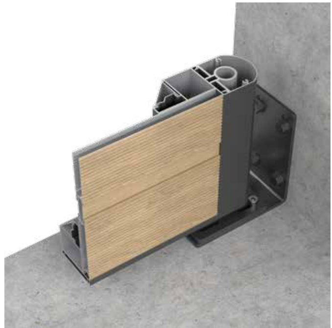
Detailed views of the sash and grooved profiles, along with the pivot axis profile with INOX 316 PIN able to hold 250 kg each. Maximum single door sash is close to 4m 2 withstanding a maximum wind load of 2KPa.
